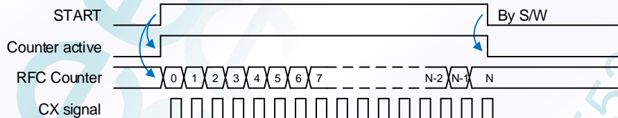
Figure 2.8: The Sample of the RFC Counter Controlled by the START Bit (RFCMOD = 1)
